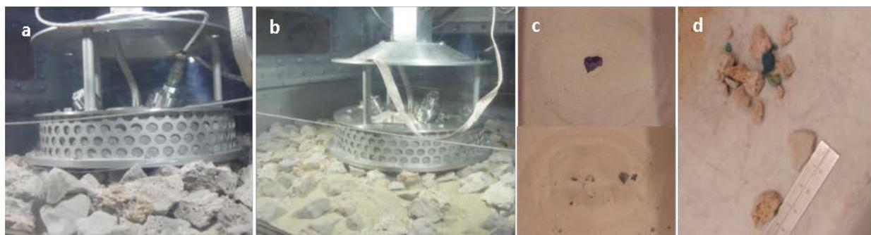
Figure 5 MPRISM October test series. (a) Test set 1 with coarse pumice pieces on top of sand layer; (b) Test set 2 with mixed coarse pumice pieces and sand; (c) Test set 3 with >3 cm piece of Allende resting on sand layer, above before sampling, below after sampling with meteorite piece completely shattered; (d) Large pumice pieces collected in Test Set 2 (inch ruler for scale).
