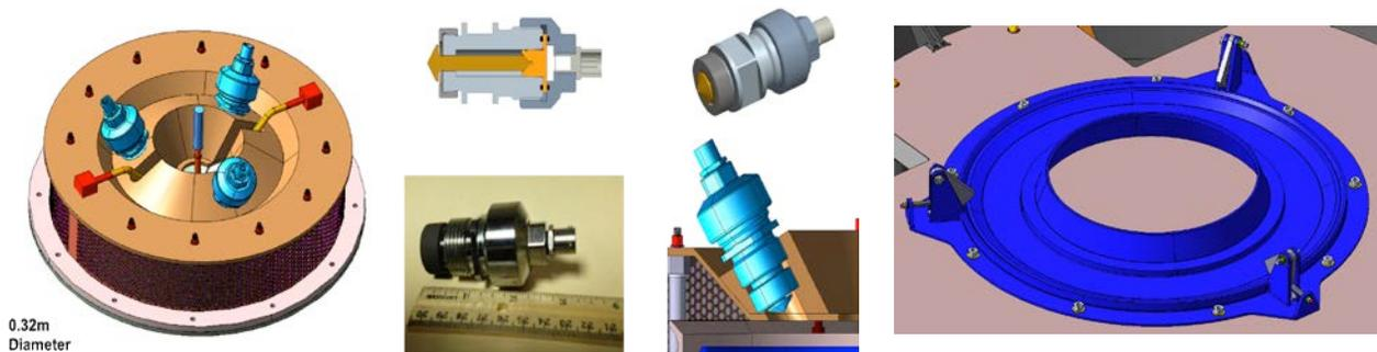
Figure 1: TAGSAM sampler integrated with 3 rock chippers (left); rock chipper (4 views, center); sample head capture ring (right), the mechanical interface to the Earth Re-entry Capsule for MPRISM. These are simple and reliable mechanisms.
