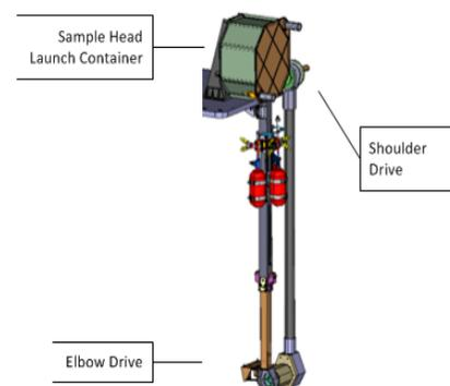
Figure 2: Sample acquisition assembly, identical to OSIRIS-Rex design.
