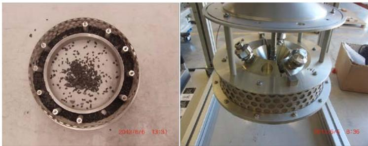
Figure 3. MPRISM sample collection test results with Mix 7C Basalt (left); integrated MPRISM sampler test fixture (right). MPRISM increases sample collection from regolith simulant and enables sampling of hard targets without loose regolith.
